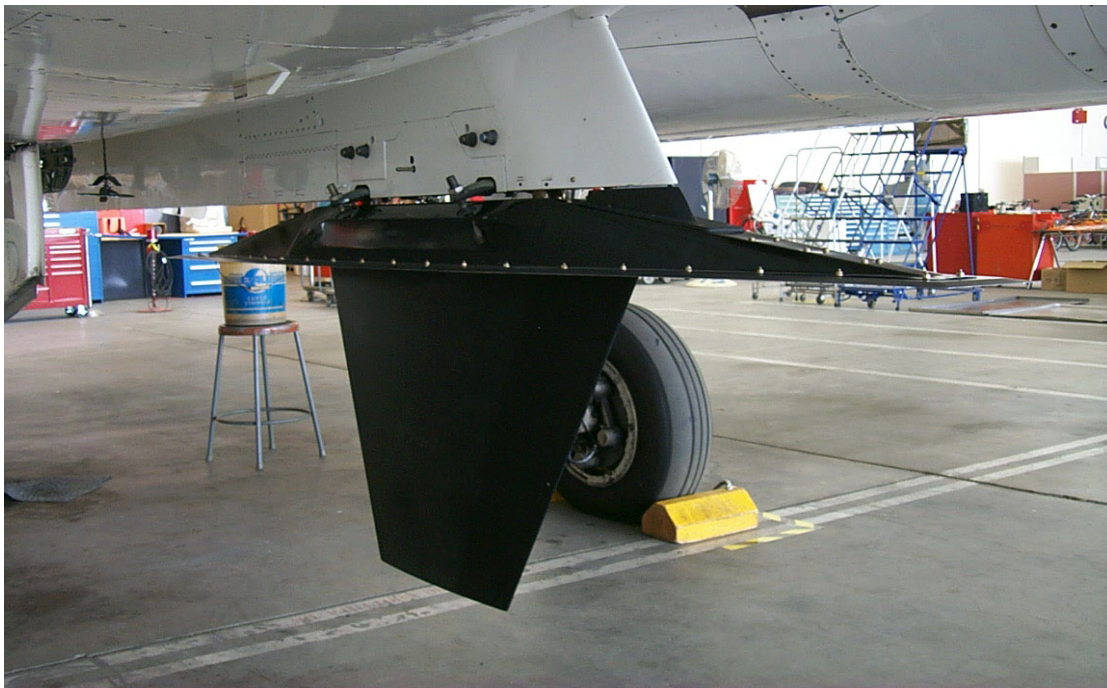
Figure 1: 30° leading-edge-sweep model under the F-15
